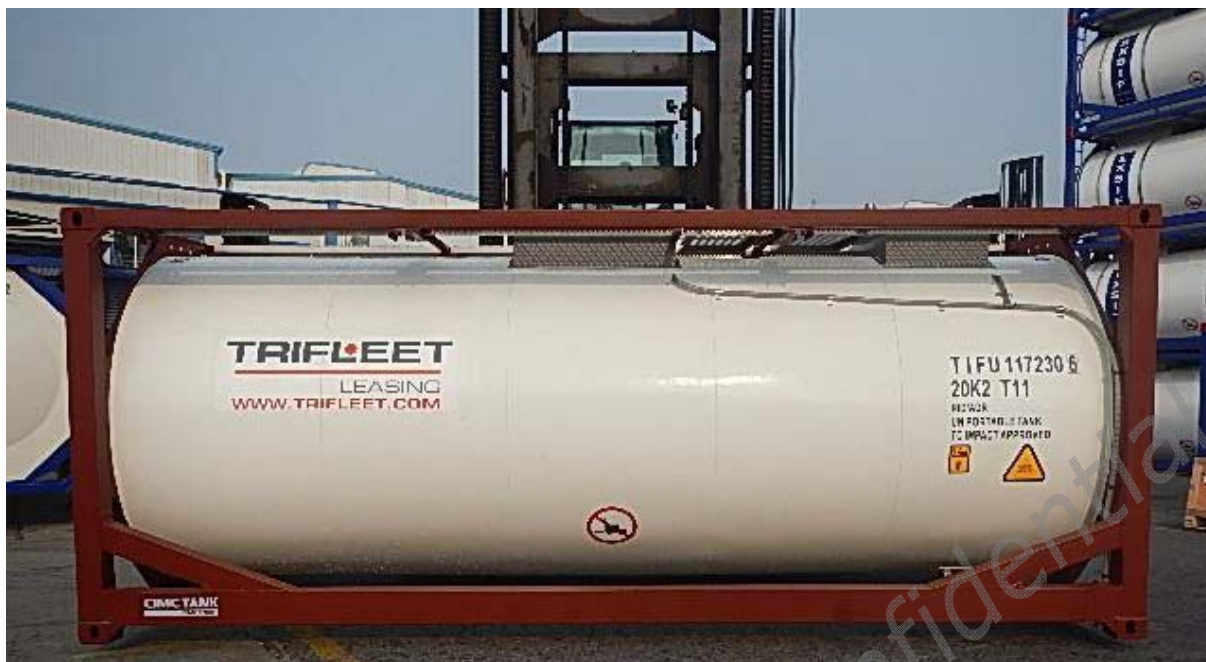
17500 Liter – UN Portable T1-T23 –Tank container
